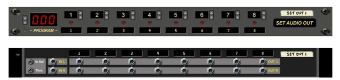
The Rack Extensions "Set Audio Out" allows you to route the signal from the In to the 8 Out. The program is selected with the "Switch Up Down Prg", while the relative 8 Out is enabled with the "Switch Up Down Set". When the "In Cv" (mode slave) is connected, the program change takes place through this connection, while the "Switch Up Down Prg" is disabled. The same signal as applied to the "Cv In" comes out of the "CV Thru".
