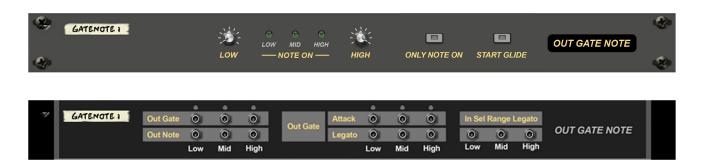
The "Out Gate Note" Rack Extensions is a monophonic generator with "Out Gate" and "Out Note". The "Only Note On" selection works on the legato and limits the notes on output only when the keys are pressed, while when they are released there will be no out event.
